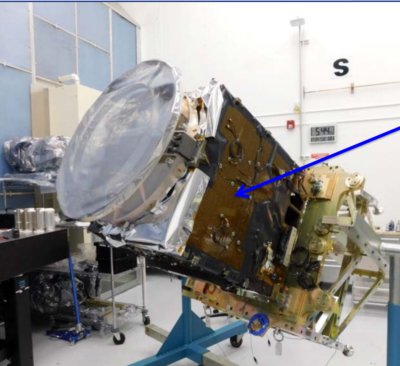
Heater panels and harnesses
